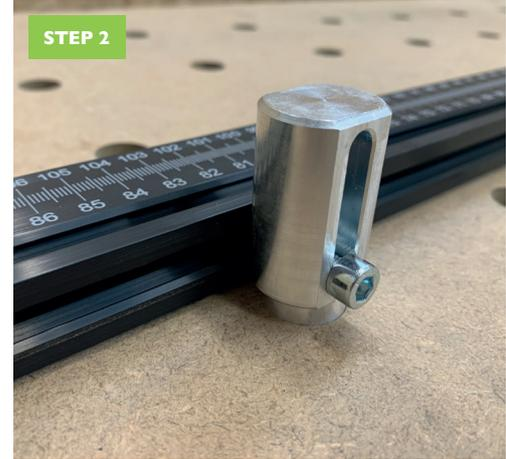
Slide the Fence Dog along the fence to desired position and place into your MFT hole.
