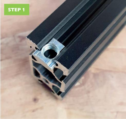
Slide the t-nut into the thin side of the fence as shown below and screw the Fence Dog into the t-nut using the low profile hex bolt.
