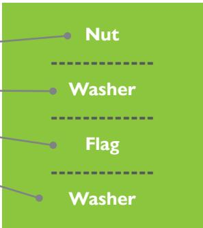
Place a washer on the bolt followed by the flag, the remaining washer and then the nut
