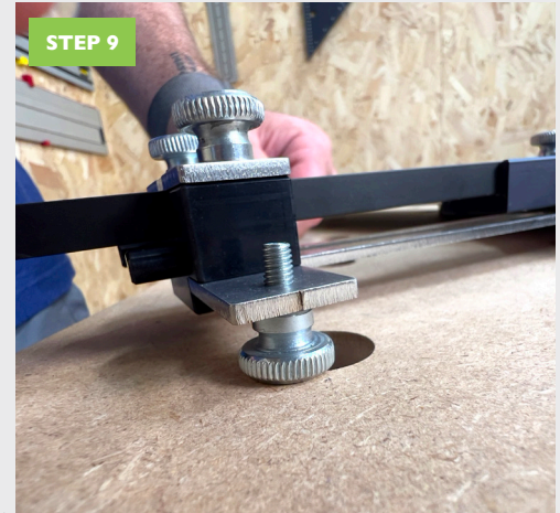
Adjust the height to suit the work piece. This will level your track and stop tilting up to 18mm
