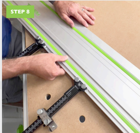
Slide track to the work piece
