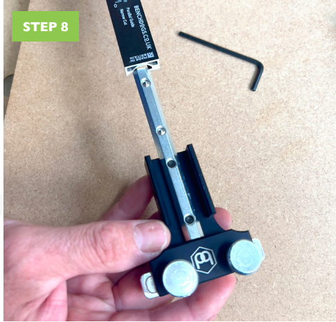
Align the fence in the slot with the joining bar
