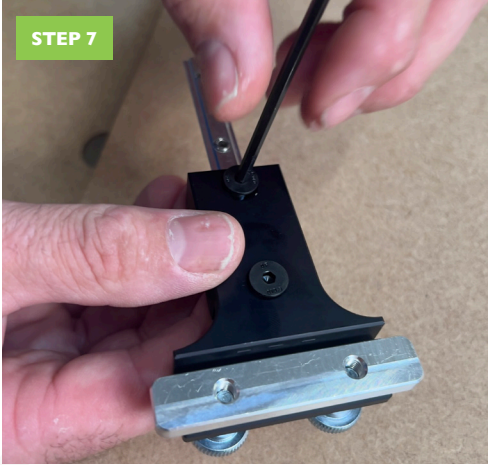
Fit M5 black screws and leave loose
