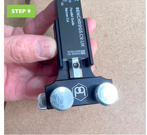
Slide in the fence in the slot to the end of the track adaptor
