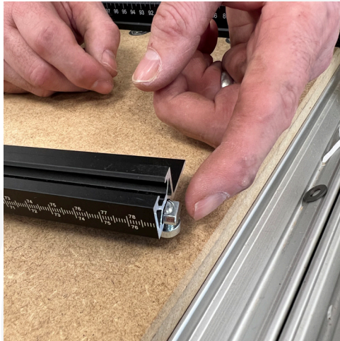
THEN SLIDE THE CALIBRATION SCREW WITH THE ATTACHED T-NUT INTO THE REPEAT STOP ON THE UNDERSIDE.
