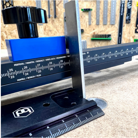
USING A RULER OR TAPE MEASURE, SLIDE IT UNDER YOUR TRACK AND BUTT IT UP TO THE FLAGSTOP.
