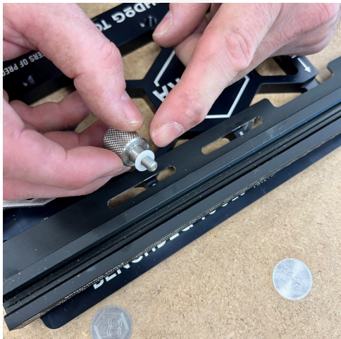
TAKE THE SUPPLIED THUMBSCREWS WITH THE PLASTIC WASHERS.
