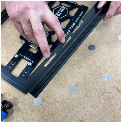
TAKE THE MK3 REPEAT STOP AND LOCATE THE LONG SLOTS WITH THE FLAT SIDE OF THE EXTRUSION FACING DOWN.
