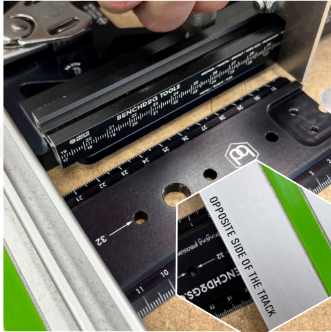
SLIDE THE REPEAT STOP TOWARDS THE TRACK AND CHECK THAT THE MEASUREMENT IS READING THE SAME MEASUREMENT ON THE RULER / TAPE MEASURE.
