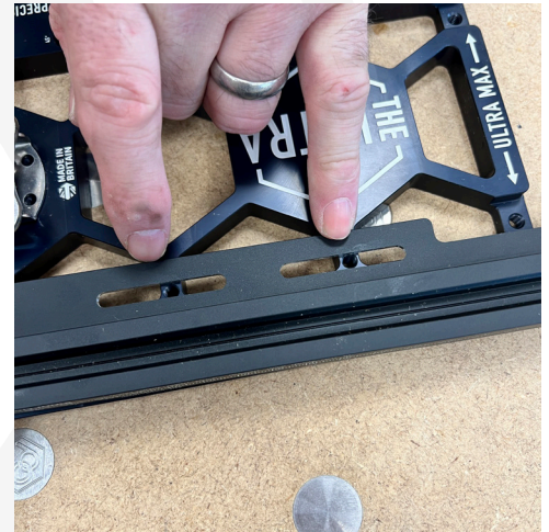
LINE UP THE REPEAT STOP SLOTS TO THE RS HOLES ON THE RAIL SQUARE
