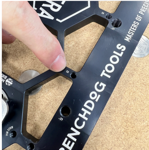
LOCATE THE RS (REPEAT STOP) HOLES
