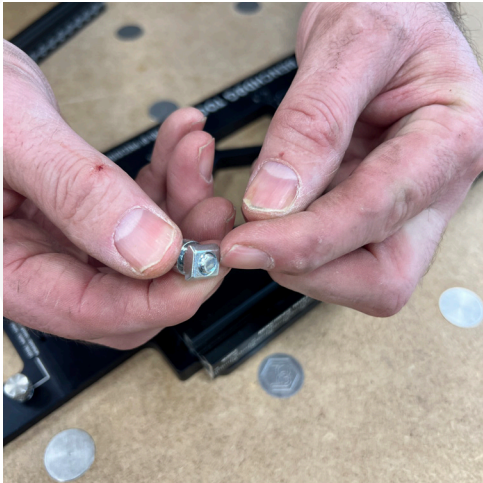
UNSCREW THE T-NUT SO IT IS TO THE TIP OF THE SCREW.
