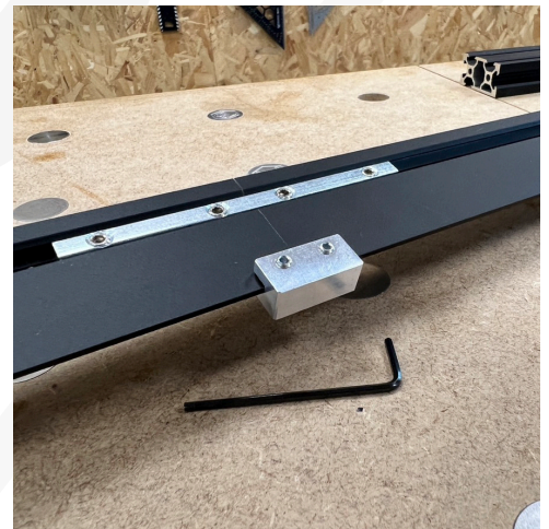
TAKING THE CONNECTOR BLOCK, YOU CAN SLIDE THIS ONTO THE EDGE, MAKING SURE ITS RIGHT IN THE MIDDLE OF THE JOIN. USING A 2MM HEX KEY YOU CAN TIGHTEN UP THE GRUBSCREWS AND THIS IS NOW SECURELY FIXED INTO PLACE.
