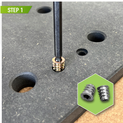
TOPSIDE OF THE MFT TOP – SCREW THE M6 SCREW NUTS INTO THE 8MM WITH 12MM RECESS HOLES WITH A M6 HEX KEY.
