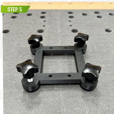
PUSH THE BENCH DOG JIG INTO THE MFT TOP USING TWO BENCH DOGS. MAKE SURE EVERYTHING IS ALIGNED.
