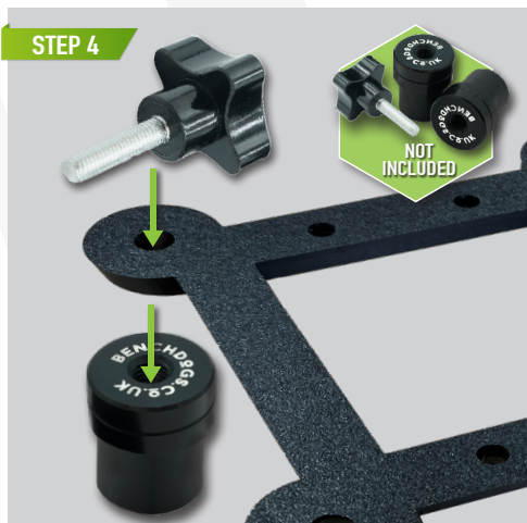
USING THE SUPPLIED BENCH DOG JIG AND 4x BENCH DOGS. PUT THE BENCH DOGS (NOT INCLUDED IN THE KIT) INSIDE THE HOLES OF THE BENCH DOG JIG AND SCREW THEM INTO PLACE USING 4x M8 THUMBSCREWS (NOT INCLUDED IN THE KIT).
